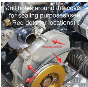
'Sealing 10' – Timing cover, belt drive
