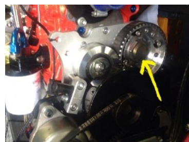
'Sealing 6' – Camshaft end nut
