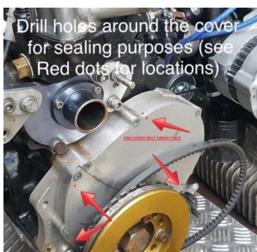
'Sealing 10' – Timing cover, belt drive
