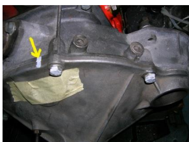
'Sealing 4' – ...flywheel / bellhousing
