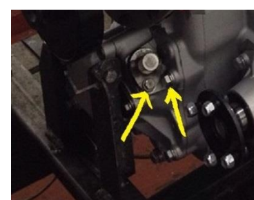
'Sealing 9' – Speedo drive/Gearbox end casing
