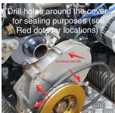
'Sealing 10' – Timing cover, belt drive
